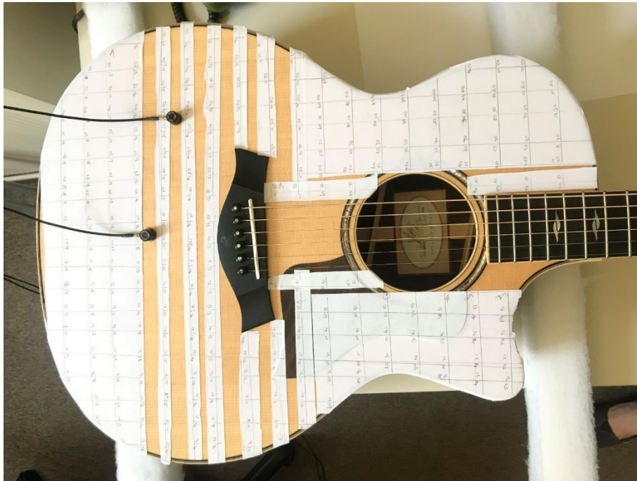
Figure 7 - Modal analysis with force hammer and two accelerometers. Accelerometers are at fixed positions and the force hammer is used for scanning the surface.
