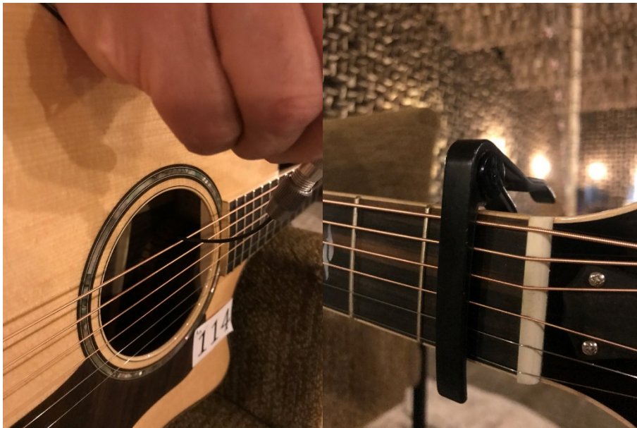
Figure 24 – Manual plugging of single notes using a helper tool made of spring steel wrapped in an insulating hose.
