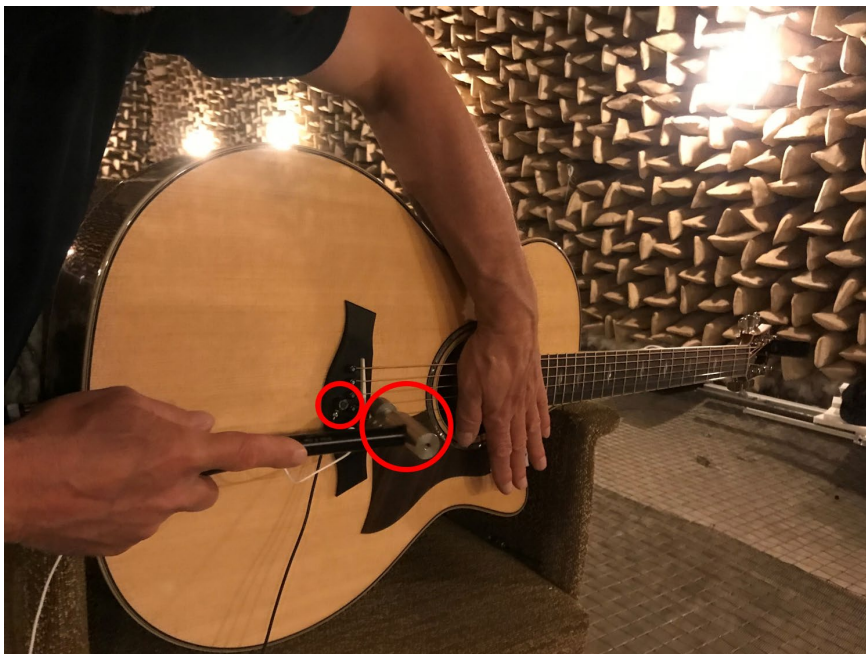
Figure 11 – Excitation of the bridge using an impact hammer with a force sensor.
