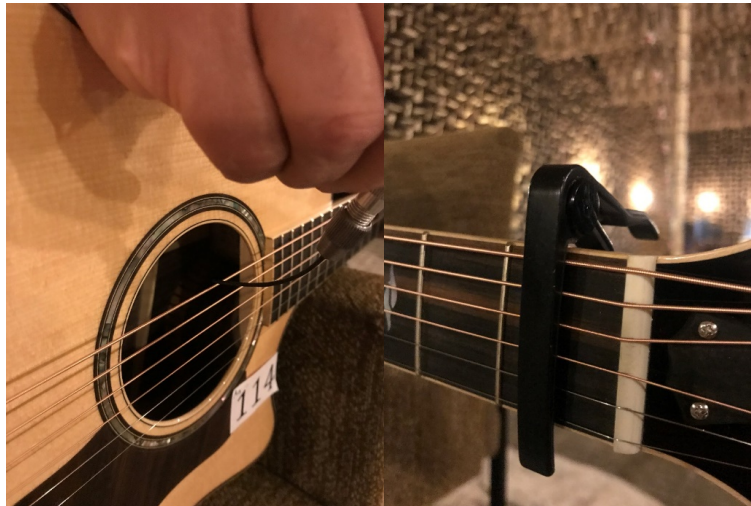
Figure 15 – Manual plugging of single notes using a helper tool made of spring steel.
