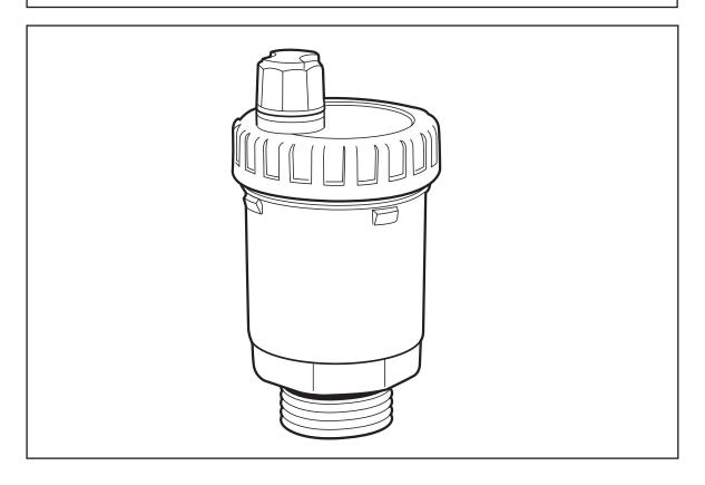
A 1/2" or 3/8" combination automatic air vent for use with sealed heating systems.
