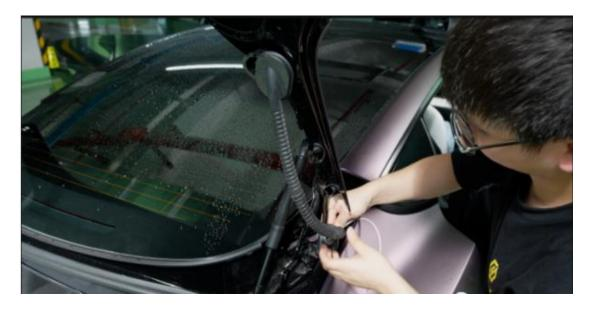
11, Note: remove the original rear camera bracket without removing the original rear license plate holder, lightly press the license plate, you can remove the original camera bracket.
