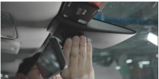
10, Rear camera wiring, following the original wiring harness wiring.
