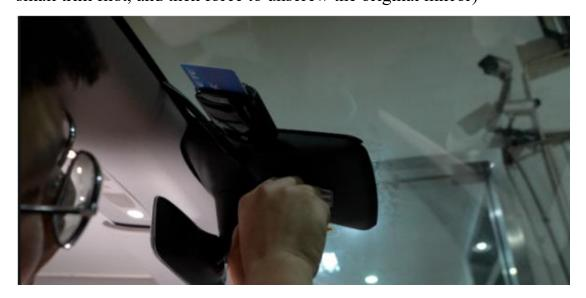
9, Replace the original mirror for installation, note that the Tesla 3/Y with the goods, the mirror bottom bracket is different.
