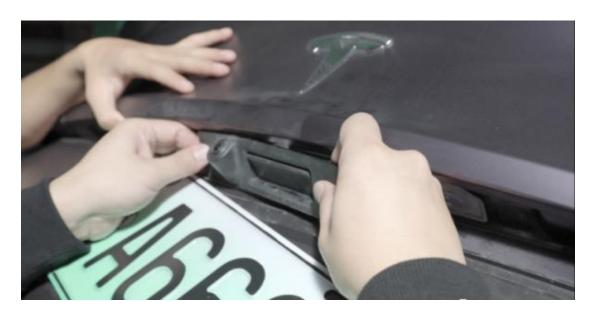
12. The chassis camera extension cable goes down from the waterproof tape, without removing the rear bar
