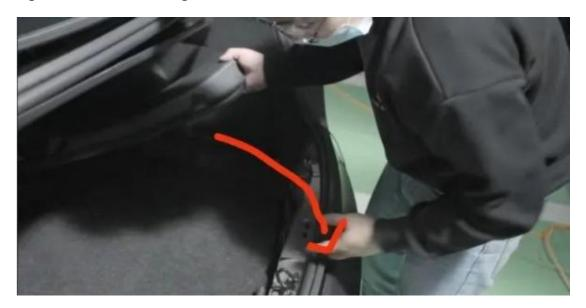
13. Route the extension cable to the middle of the vehicle, pay attention to the wiring harness not to be pressed by the bottom shield, which may cause the chassis camera not to work
