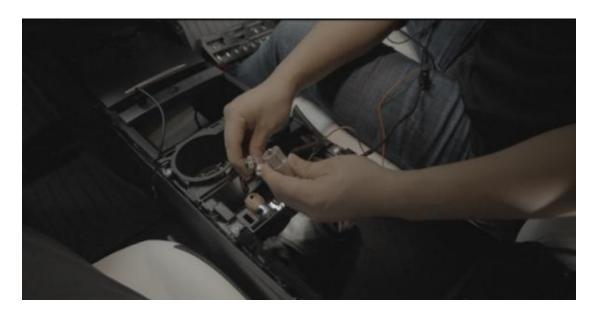
4, Removing the rear air outlet
