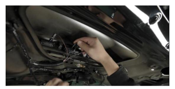
(Note: remove the original rear camera bracket without removing the original rear license plate frame, lightly press the license plate, you can remove the original camera bracket)
