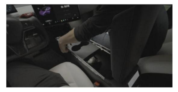
3, Find the original cigarette lighter plug under the water cup holder, and transfer the plug to take the power
