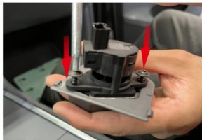
19 Lock The Removed Temperature Sensor Into The Matching Heat Dissipation Plate And Fasten It With M4 Screw
