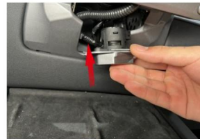
21 Clip The Installed Sensor Into The Cover
