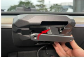
10 Install The Upper Cover Trim Panel (the Bracket Has Been Rotated By 40 And Can Be Directly Installed)
