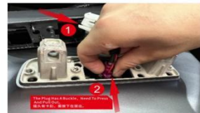
6 Remove The White Clip First And Then Pull The Plug In Sequence
