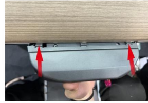
12 Snap The Cover Into Place (be Careful Not To Drop The Fastening Strip)
