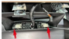
5 Remove The Two Screws With T27. And Put The Original Car's Removal Of Screen Cover
