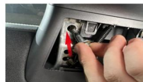
3 Remove the two screws of the original car with the No. 10 wrench
