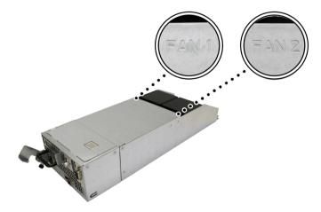
3 Find the malfunctioning fan. Lift the fan upward to remove it.
