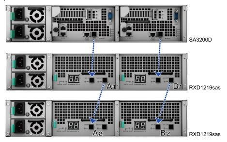
**4** Connect one end of the power cord(s) to the power port of RXD1219sas, and the other to the power outlet(s). RXD1219sas will automatically power on once the power cords are correctly connected.
