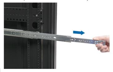
3 Align the fixing holes of the inner rail to the side of the chassis and slide backward to attach the inner rail.
