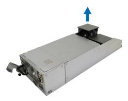
4 Prepare a new fan, and slide it into the controller. Make sure the fan is properly slide in.
