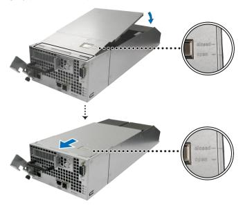
**d** Insert the controller back in SA3200D. Push back the release lever and turn the screw clockwise to secure the controller.
