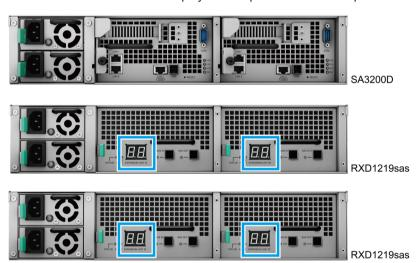
**Note:** Even with the Synology NAS and expansion unit(s) powered on, you can still expand with one or two expansion unit if needed. To do so, repeat above steps to connect the expansion cables and power cords of the other expansion units. Your expansion units will automatically power on if they are correctly connected, and the expansion unit ID will be displayed accordingly after a few seconds (if DSM is correctly initialized in the Synology NAS server).
