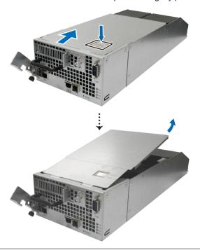
**Note:** When you remove the rear top cover, the sensitive internal components are exposed. Avoid touching anything other than the memory assembly when you remove or add memory.
