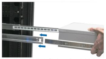
5 Pull and hold the front latch of the inner rail to unlock the inner rail, and push the chassis towards the rack. Use the cage nuts and screws in the rail kit package to secure the chassis to the rack if necessary.
