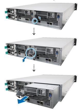
3 Press the release button on the rear top cover. Slightly push backward to lift the rear top cover.
