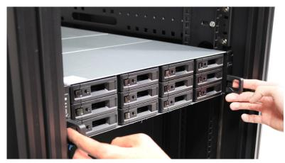
2 With the help of another person, carefully remove the chassis from the rack. Then, slide the inner rail attached to the chassis toward the front panel of the chassis to detach it.
