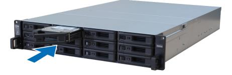
Note: Make sure that the drive tray is completely inserted. Otherwise, the drive might not function properly.
