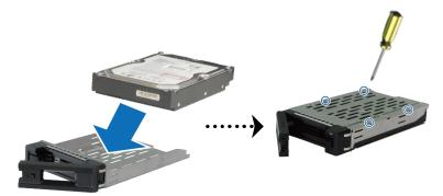
• For 2.5" drives: Place the drive in the drive tray. Turn the tray upside down and tighten screws into the four spots indicated below to secure the drive in place.
