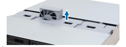
**5** Prepare a new fan and slide it into the your RS3621xs+. Make sure that the fan is aligned properly, as shown below.
