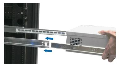
**5** Pull and hold the blue front latch of the inner rail to unlock the inner rail. Push the chassis into the rack. Use the cage nuts and screws enclosed with the rail kit package to secure the chassis to the rack if necessary.
