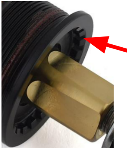
Bottom Bracket: Bottom bracket teeth that can be damaged of #10-32 flat head screws are not installed with enough torque
