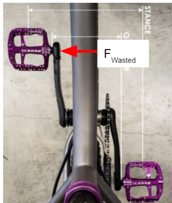
Figure 5: Direction of wasted force on a crank
