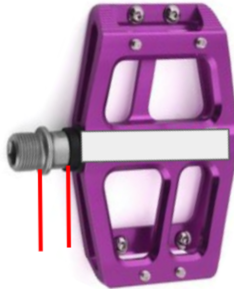
Figure 2B: Pedal with short axle length
