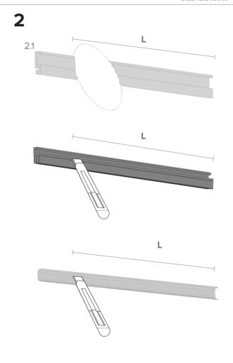
**2.1** Measure the full width of the door (L) and cut aluminium holder to required length, file off any rough edges. Cut the rubber insert and cover cap to the same size.
