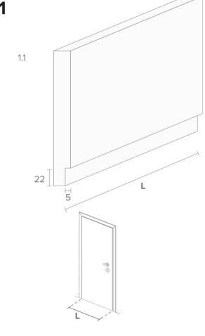
**1.1** Remove the door from the hinges and lay on its side then restrain firmly. route a groove 22mm x 5mm deep the full length of the door (L)
