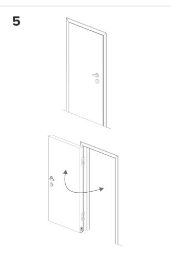
**5** Open and close door to test seal drop.
