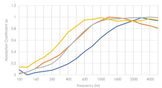
University of Auckland Test Report Number Frequency (Hz) 125 250 500 1000 2000 4000 NRC α<sub>P</sub> 12mm Cube T0712-3 0.05 0.10 0.30 0.65 0.90 0.95 0.45 α<sub>P</sub> 12mm Cube (with 25mm air gap) T0712-6 0.05 0.30 0.60 0.95 0.95 0.85 0.70 α<sub>P</sub> 24mm Cube 0.90 1.00 1.00 0.70 αρ 24mm Cube rith 25mm air ga 0.40 0.80
