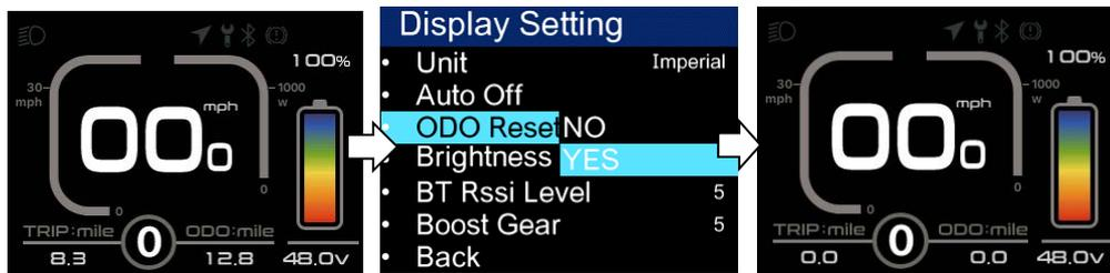
On the main interface, press and hold the "+" and "-" keys at the same time to achieve zero TRIP and AVG, as shown in the following figure:
