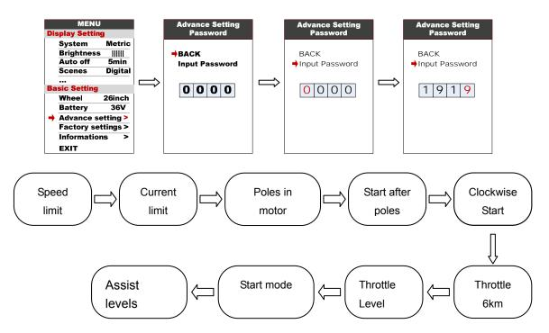
**8.12 Speed limit**: Press UP/DOWN will change speed limit, range 10km/h~45km/h. Default value is 25km/h.
