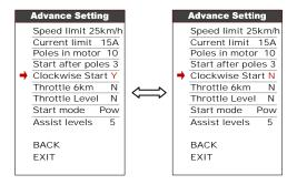
**8.17 Throttle 6KM**: this parameter can set the throttle function, N represent max speed, Y represent 6Km.
