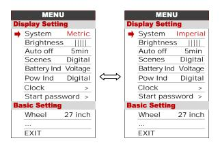
**8.2 Brightness**: Press Up / Down button to change the brightness of the backlight, i is darkness, iiii is brightness
