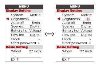
**8.3 Auto off :** Press UP/DOWN button to change the auto power off time, from 1 to 9, the number represent time (minutes) to shutdown, default value is 5 minutes.
