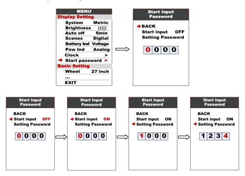
You need to input the right password before start with 30 seconds, display will power off automatically if the password was wrong.
