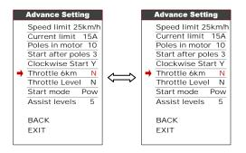
**8.18 Throttle Level**: This parameter is functional when Throttle 6KM set N, Press UP/DOWN will change Y/N, N represent Throttle start max speed, Y represent throttle's speed is accorded to the assist level.
