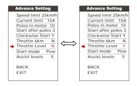
**8.19 Start mode**: Pow/ECO/STD represent Power/ECO/Standard, Power mode means use maximum current when speed up (default), ECO mode means use minimum current.
