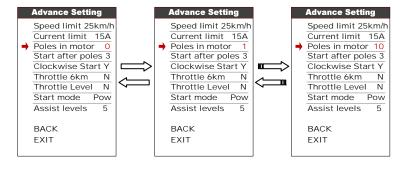
**8.15 Start after poles**: How many poles (speed sensor) need to be detected by controller before starting motor. Default value is 3.
