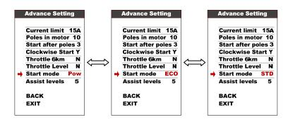
**8.20** Assist levels: This parameter can customize assist levels, options are 3/5/9/UBE, UBE represent factory default settings.
