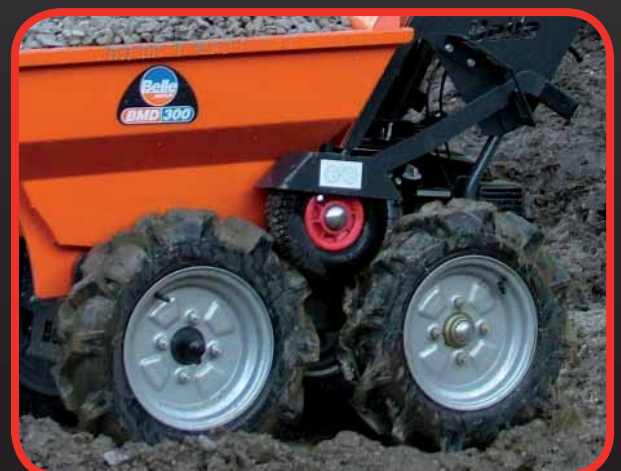
Carrier wheel disengages for easy wheel change
