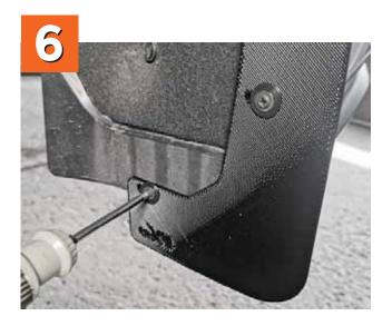
**A.** When satisfied with the position of the flap, screw one of the supplied screws(D) into the lower plastic trim of the bumper through the lower slotted hole of the mud guard.
