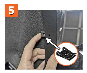
**A.** Grab one of the provided u-nuts(E) and slightly pry it open to facilitate the installation and avoid scratching the paint.
