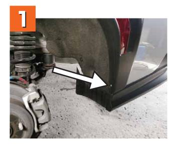
**A.** Jack you car up so you can remove the rear wheel and gain access to the bumper inner lip.
