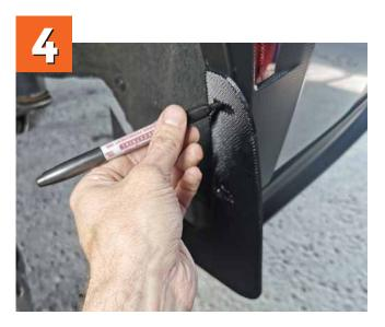
**A.** Rotate the mud guard so that the upper slotted hole aligns with the bumper. Mark the spot with a pen.
