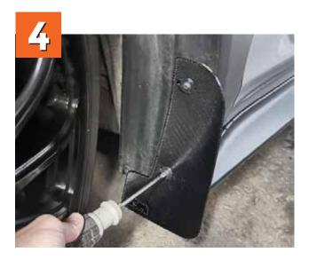
**A.** Align and screw both screws into the fender liner. Don't tighten all the way to allow positionning the flaps to your liking.
