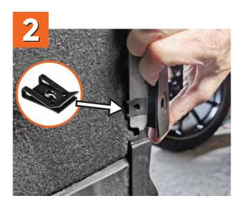
**A.** Grab one of the provided u-nuts(E) and slightly pry it open to facilitate the installation and avoid scratching the paint.
