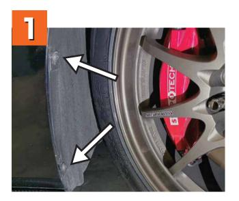
**A.** Turn your vehicle's front wheels as much as possible to allow access to the 2 factory fender liner screws.
