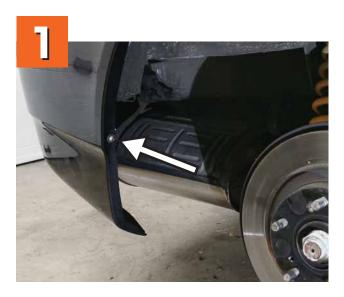
**A.** Jack you car up so you can remove the rear wheel and gain access to the bumper bolt.
