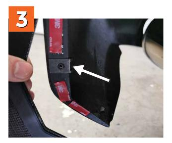
**A.** Position the rock guard roughly into position and mark the spot where the lower hole aligns with the bumper.
