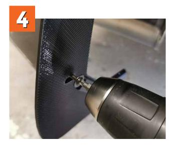
**A.** Double check the alignement of the u-nut hole. Slightly move the rock guard from left to right and decide on its final positionning.
