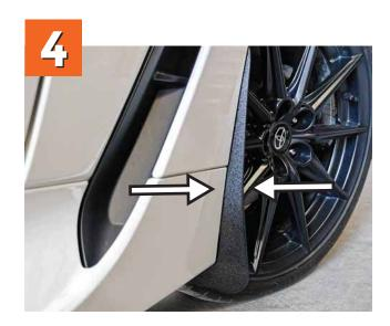
**A.** Adjust the position of the mud flaps to your liking. When satisfied, you can tighten all screws completely.
