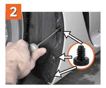
**A.** Grab 3 of the provided rubber screw grommets(E) that came in the front mud guards' package.
