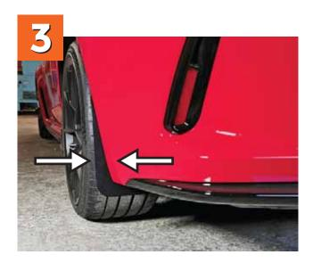
**A.** Move the rock guard from side to side to the desired position.
