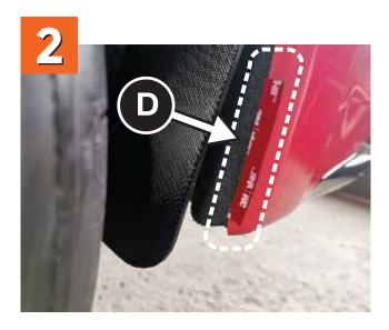
**A.** Rotate the rock guard to expose the bumper inner lip.
