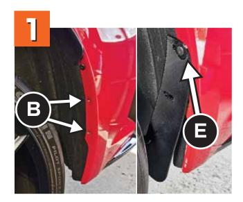
A. Jack your car up so you can remove the rear wheel and gain access to the bumper inner lip. If you have a small enough screwdriver, this step is not required.
