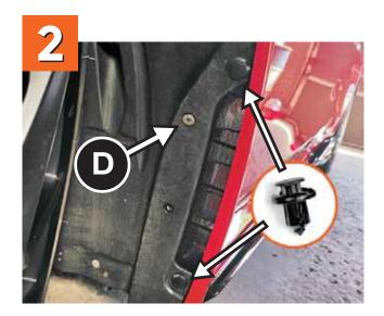
A. Align both holes with the fender tab holes and squeeze the taller edge of the mesh into the fender inner lip.
