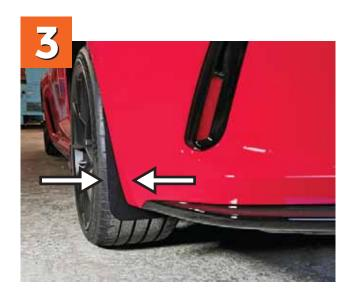
**A.** Move the mud guard from side to side to the desired position.
