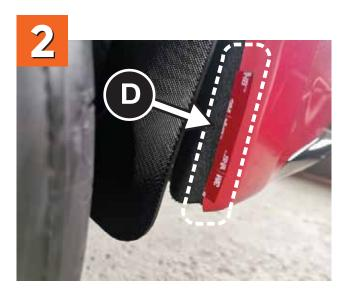
**A.** Rotate the mud guard to expose the bumper inner lip.
