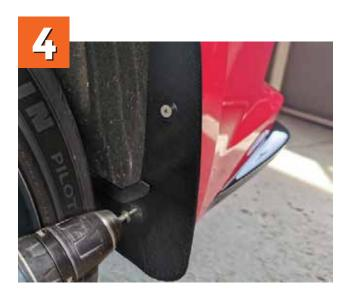
**A.** Grab one of the provided 1" (25mm) Phillips flat head screw (F) and one of the 3/16" (5mm) spacer(G).
