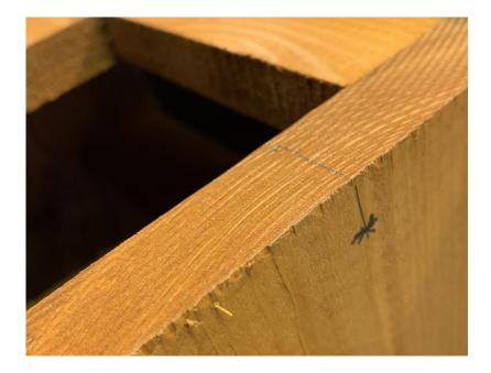
From the line, mark a point approximately 6mm in from the edge (as shown above) and drill a 4.5mm hole, taking care to keep the drill straight. The hole needs to be 4.5mm to give grip to the hinge pin.
