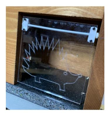
The rod then needs to pushed into place keeping the door parallel with the opening. It's a bit fiddly but it is important you get the position right else the door will not swing easily.
