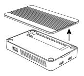
Attach the thermal pad on the top of SSD. Then slide the SSD at 45° into the slot until it is fully seated.
