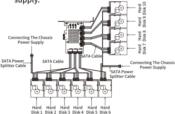
3. Reconnect all the power cables to start up the computer, then install the ACASIS PCIe 10-port SATA expansion card driver. Please download the driver from ACASIS website: www.acasis.com
