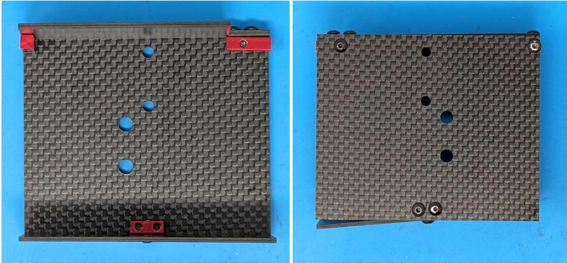
**Step 03)** Using 4-40 x 7/16" screws attach 1 piece of corner nutstrip to each sidewall. Be sure to note orientation. You want them on the inside of the walls with the threaded hole facing up. The top hole is for the lid.
