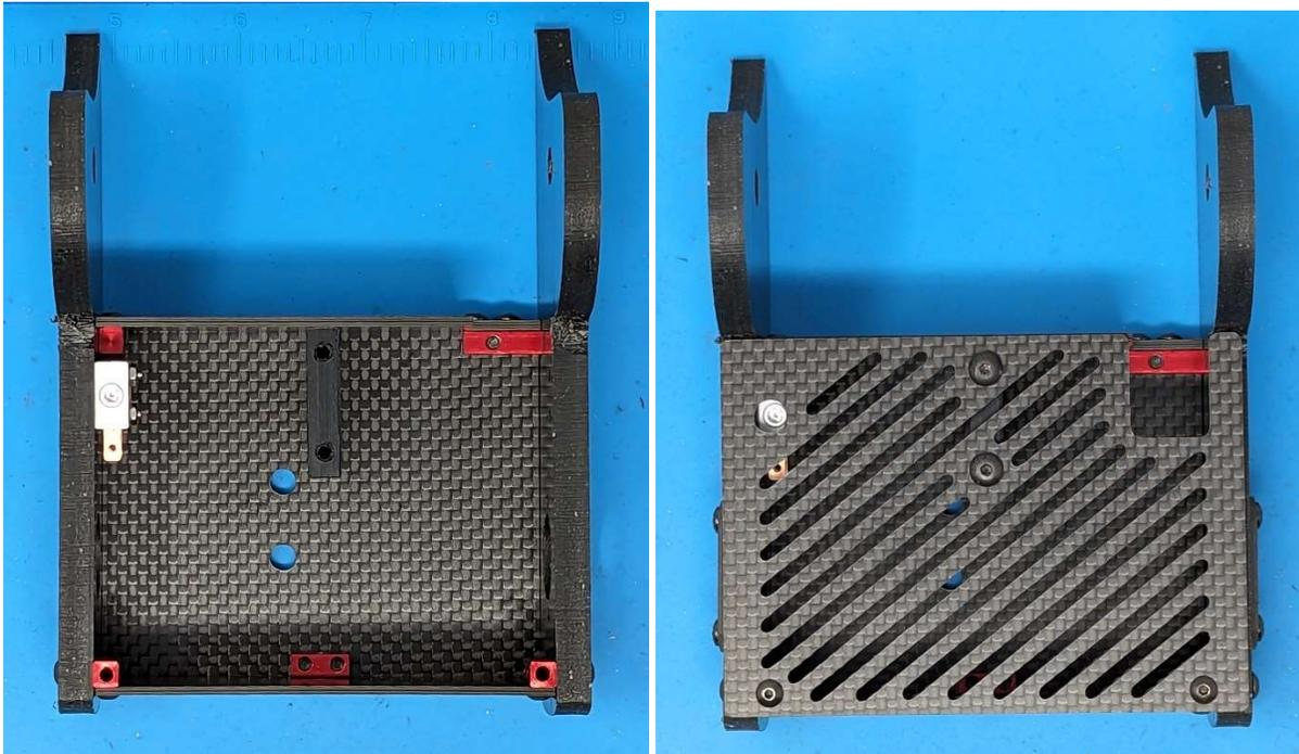
**Step 06)** Install Drive Motor Plates using the 4 Plastite Phillips Screws. Two for each side.
