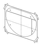
Drill 1/4" (6mm) diameter holes through the markings provided on the template. There is no need to find a stud in your wall. Be as precise as possible.
