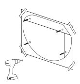
Remove template from the wall. Choose the appropriate anchor based on the material of your wall. Insert anchors into drilled holes. Anchor must be flush with the wall!
