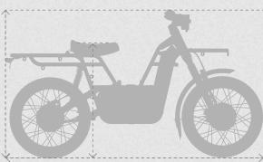
LENGTH: 1.8m | 6ft WIDTH: 0.84m | 33in WHEELBASE: 1.2m | 4ft **HEIGHT:** 1.02m | 3.37ft SEAT HEIGHT: 0.8m | 32in
