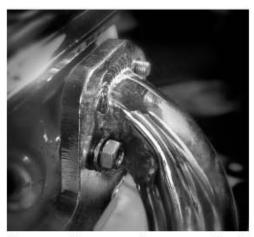
Some studs cannot be accessed with a socket. The nut and washer should be started before the header is fully tightened down. Number 2 shown.
