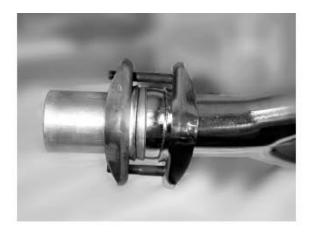
We utilize the popular ball and socket style of exhaust flange. It is important to alternate between the 2 bolts as you tighten them so that they are tightened evenly and equally. We also recommend that you use a jam nut on the bolts to keep them from loosening due to vibration.
