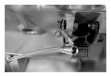
Now you can install both left and right side headers from the top down. Some studs cannot be accessed with a socket. The nut and washer should be started before the header is fully tightened down, as shown below.
