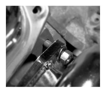
Once the headers are in place, tighten from the middle outward to gasket manufacturers specs.
