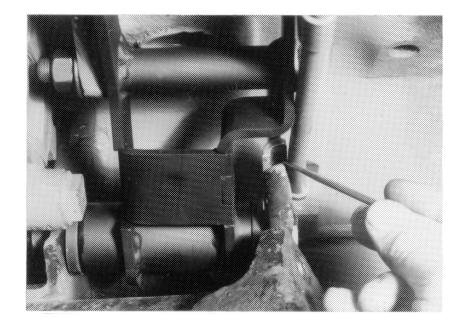
You should have enough room for the dipstick tube to be installed (as showed above). If more clearance is needed, you can grind on the K-Member perch for clearance.
