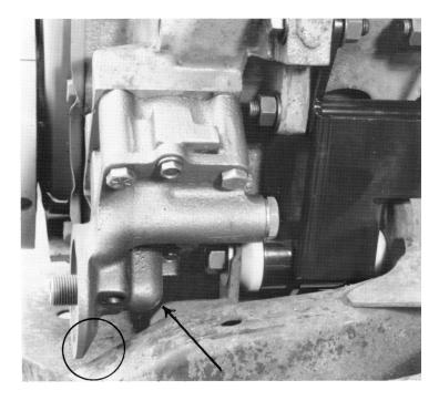
With a Melling or high volume oil pump and additional notch and material removal may be required (see picture above). The notch for the oil filter starts approximately 3 inches in front of the perch. At times it may be necessary to elongate the 9/16" hold or use a 7/16"x5" Grade 8 bolt to allow for greater adjustability.
