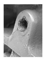
You will need to drill and tap two 1" deep holes for the bracket. For the average street car use tap size 3/8" x 16 (course) with a drill size of 5/16". For more performance oriented vehicles use tap size 7/16" x 14 (course) with a drill size of "U" or 25/64". Drill a pilot hole in the center of your scribed mark. I use a piece of tape to mark the depth. (1")
