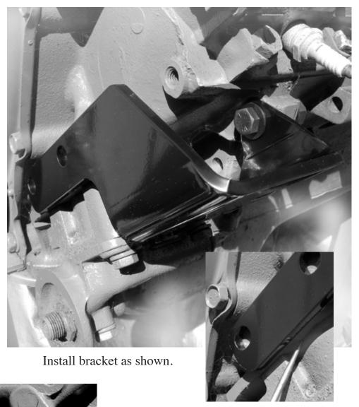
Line up bottom of the bracket to the bottom edge of oil pump. (see scribe)
