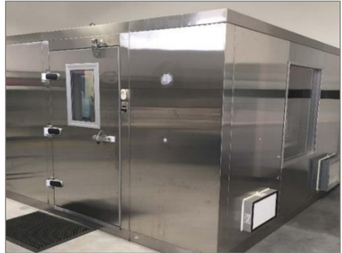
Figure 2: Exterior picture of the Stainless Steel Bioaerosol Test Chamber used for all P3000 Testing. Chamber is equipped with HEPA in/out, multiple bioaerosol sampling ports, decontamination, temperature and humidity control, and pressure balance.
