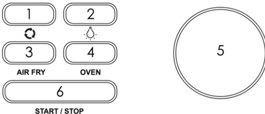
1. **Rotate:** Use when cooking with the rotisserie spit. Press the Rotate button to turn on the rotisserie mode and make the accessory rotate to achieve an evenly crispy outcome. Press again to turn off the rotisserie function. The Rotisserie function can be activated/inactivated at any time during the cooking process. The rotate button and icon will turn on when activated.
