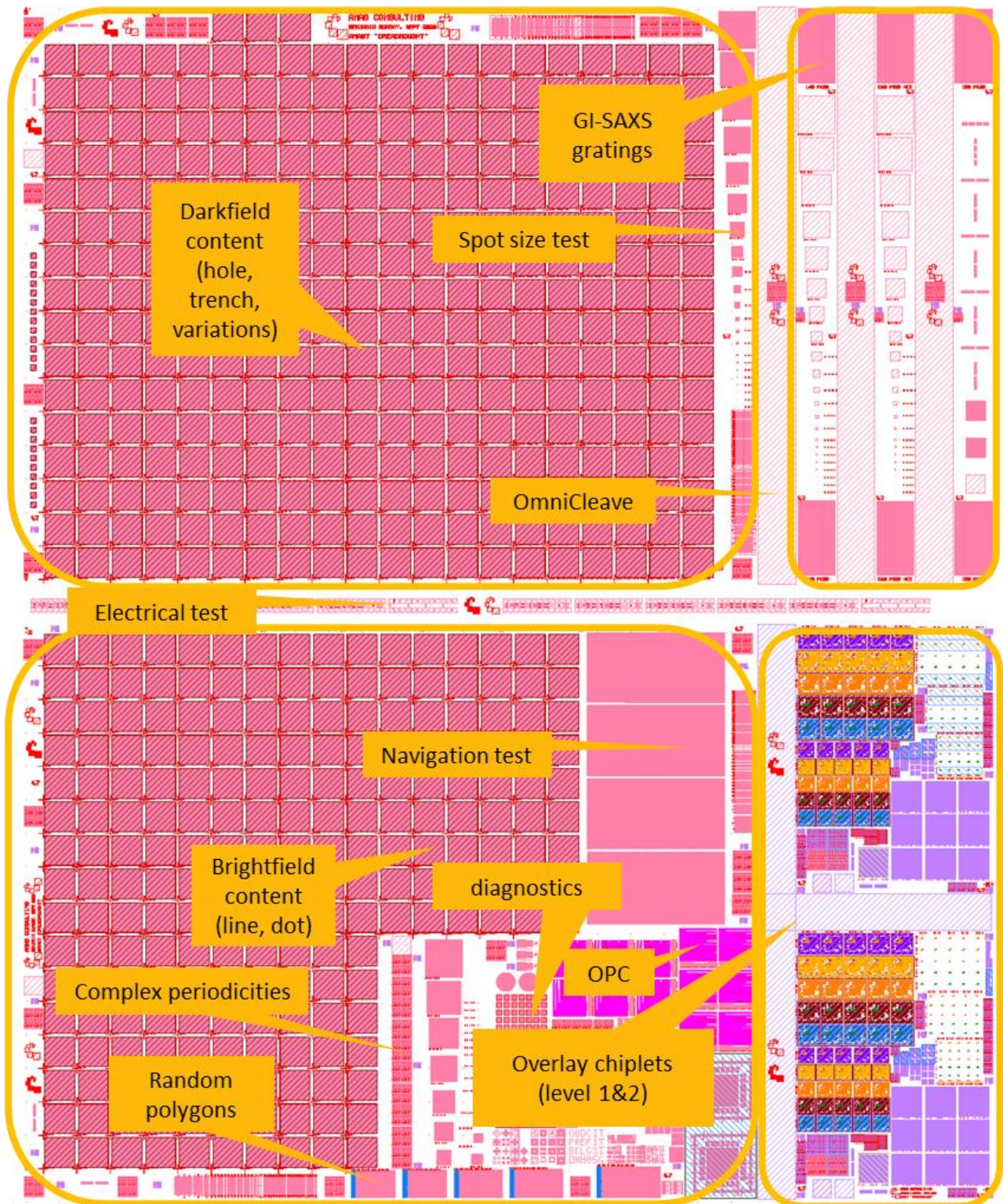
Figure 1. AMAG7 floorplan, marking some of its key features. Reticle is full standard 26 x 32 mm field size.
