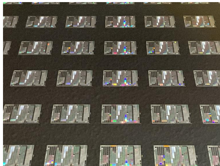
Photograph of HARhole pattern (rough pattern between die is just reflection off ceiling)
