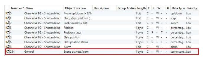
Alarm: If it receives a "0" it starts to count the "monitoring period" or executes the action that is configured in the behaviour parameter. Each time it receives a "0", the time is preloaded again. In the case that it doesn't received another "0" and the monitoring time is exceeded, it executes the alarm or the programmed alarm action. If it receives a "1", it executes the programmed alarm action.
