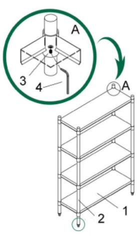
Adjust leg height to level shelving unit after assembly
