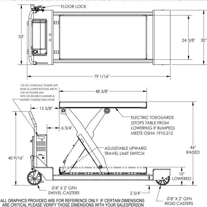
DIMENSION TOLERANCE ± 1/2" TABLE HEIGHT TOLERANCE ± 1/2" DECK FLATNESS ± 1/4"
