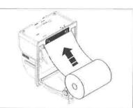
Remove the existing paper roll. Position in the correct direction, as shown above.
