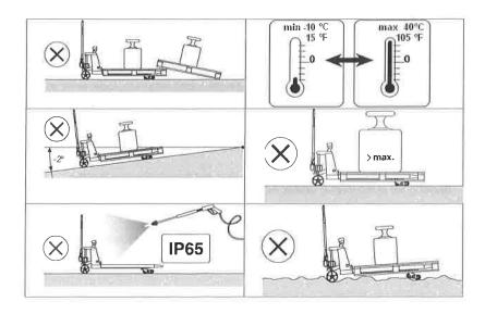
Fast temperature changes should be avoided because condensation may form in the electronics. During acclimatization the indicator must be turned off.
