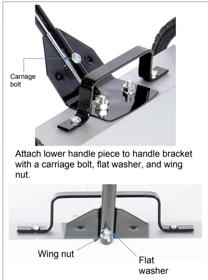
Attach lower handle piece to handle bracket with a carriage bolt, flat washer, and wing nut.
