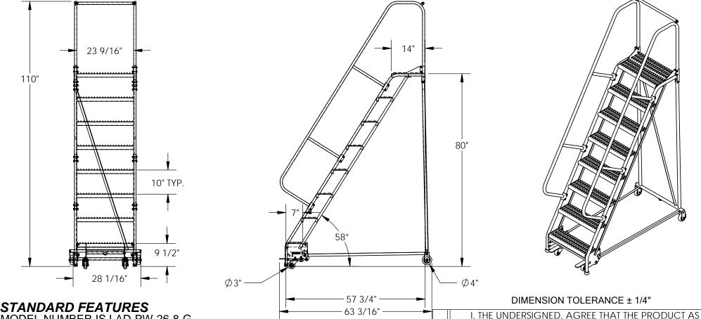
STANDARD FEATURES MODEL NUMBER IS LAD-PW-26-8-G OVERALL WIDTH IS 28 1/16" USABLE WIDTH IS 23 9/16" **OVERALL LENGTH IS 63 3/16" USABLE LENGTH IS 57 3/4" OVERALL HEIGHT IS 110"** PLATFORM HEIGHT IS 80" STEP TYPE IS GRIP STRUT CLIMB ANGLE IS 58° STEP DEPTH IS 7" PLATFORM DEPTH IS 14" **COLOR IS VESTIL BLUE BOTTOM STEP COLOR IS YELLOW** MAX CAPACITY IS 350 LBS FRONT WHEEL IS SWIVEL, SIZE IS Ø 3" REAR WHEEL IS RIGID, SIZE IS Ø 4"
