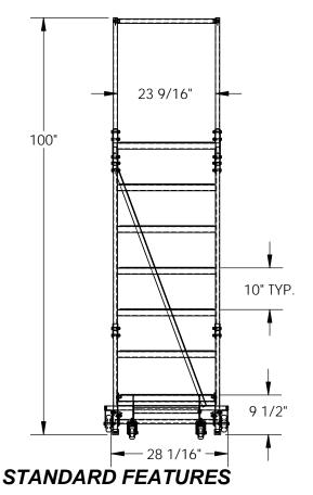
MODEL NUMBER IS LAD-PW-26-7-P OVERALL WIDTH IS 28 1/16" USABLE WIDTH IS 23 9/16" **OVERALL LENGTH IS 56 5/16" USABLE LENGTH IS 51 1/2" OVERALL HEIGHT IS 100"** PLATFORM HEIGHT IS 70" STEP TYPE IS PERFORATED CLIMB ANGLE IS 58° STEP DEPTH IS 7" PLATFORM DEPTH IS 14" **COLOR IS VESTIL BLUE BOTTOM STEP COLOR IS YELLOW** MAX CAPACITY IS 350 LBS FRONT WHEEL IS SWIVEL, SIZE IS Ø 3" REAR WHEEL IS RIGID, SIZE IS Ø 4"
