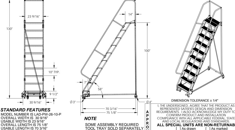
OVERALL WIDTH IS 30 9/16" USABLE WIDTH IS 23 9/16" OVERALL LENGTH IS 75 1/8" **USABLE LENGTH IS 70 3/16"** OVERALL HEIGHT IS 130" PLATFORM HEIGHT IS 100" STEP TYPE IS PERFORATED CLIMB ANGLE IS 58° STEP DEPTH IS 7" PLATFORM DEPTH IS 14" **COLOR IS VESTIL BLUE BOTTOM STEP COLOR IS YELLOW** MAX CAPACITY IS 350 LBS FRONT WHEEL IS SWIVEL, SIZE IS Ø 3" REAR WHEEL IS RIGID. SIZE IS Ø 4"
