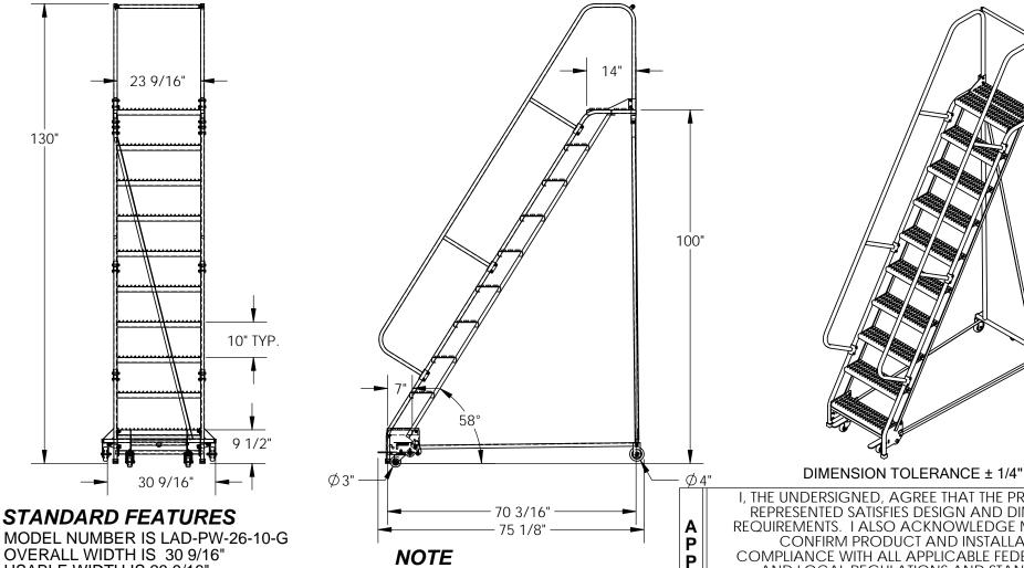
MODEL NUMBER IS LAD-PW-26-10-G OVERALL WIDTH IS 30 9/16" USABLE WIDTH IS 23 9/16" **OVERALL LENGTH IS 75 1/8" USABLE LENGTH IS 70 3/16"** OVERALL HEIGHT IS 130" PLATFORM HEIGHT IS 100" STEP TYPE IS GRIP STRUT CLIMB ANGLE IS 58° STEP DEPTH IS 7" PLATFORM DEPTH IS 14" **COLOR IS VESTIL BLUE BOTTOM STEP COLOR IS YELLOW** MAX CAPACITY IS 350 LBS FRONT WHEEL IS SWIVEL, SIZE IS Ø 3" REAR WHEEL IS RIGID. SIZE IS Ø 4"
