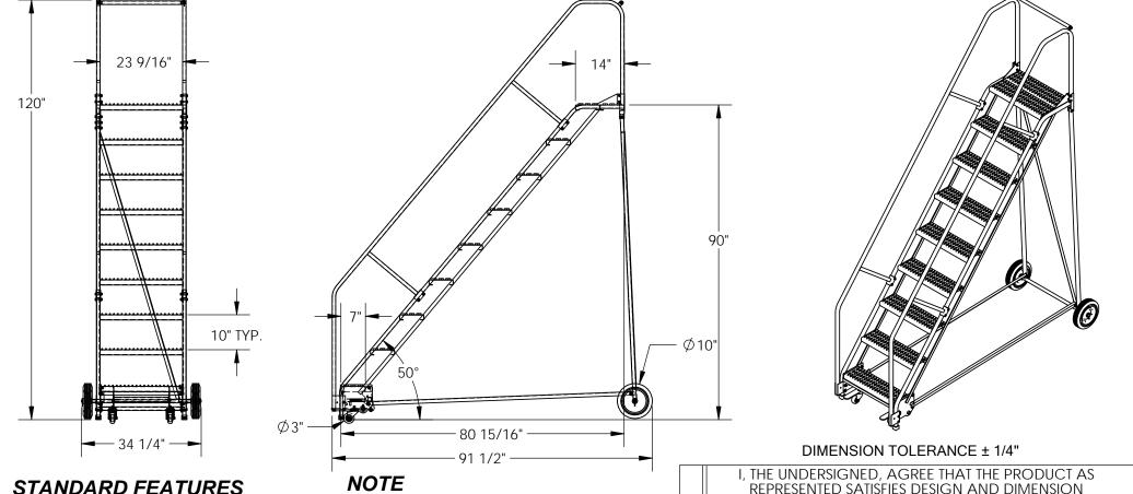
MODEL NUMBER IS LAD-9-14-G-EZ OVERALL WIDTH IS 34 1/4" USABLE WIDTH IS 23 9/16" OVERALL LENGTH IS 91 1/2" USABLE LENGTH IS 80 15/16" OVERALL HEIGHT IS 120" TOP STEP HEIGHT IS 90" STEP TYPE IS GRIP STRUT CLIMB ANGLE IS 50° STEP DEPTH IS 7" TOP STEP DEPTH IS 14" MAX CAPACITY IS 350 LBS WHEEL SIZE IS Ø10" FRONT WHEEL SIZE IS Ø3" POWDER COAT FINISH
