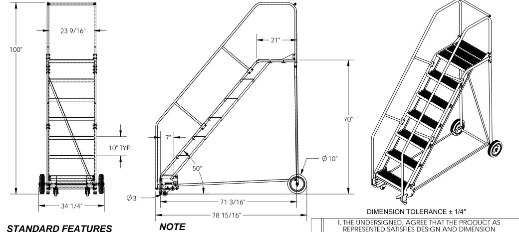
MODEL NUMBER IS LAD-7-21-P-EZ OVERALL WIDTH IS 34 1/4" USABLE WIDTH IS 23 9/16" **OVERALL LENGTH IS 78 15/16" USABLE LENGTH IS 71 3/16" OVERALL HEIGHT IS 100"** TOP STEP HEIGHT IS 70" STEP TYPE IS PERFORATED CLIMB ANGLE IS 50° STEP DEPTH IS 7" TOP STEP DEPTH IS 21" MAX CAPACITY IS 350 LBS WHEEL SIZE IS Ø10" FRONT WHEEL SIZE IS Ø3" POWDER COAT FINISH COLOR IS BLUE, BOTTOM STEP IS YELLOW
