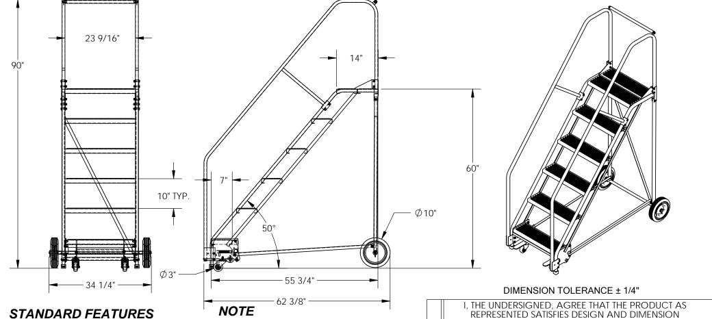
MODEL NUMBER IS LAD-6-14-P-EZ OVERALL WIDTH IS 34 1/4" USABLE WIDTH IS 23 9/16" **OVERALL LENGTH IS 62 3/8"** USABLE LENGTH IS 55 3/4" **OVERALL HEIGHT IS 90"** TOP STEP HEIGHT IS 60" STEP TYPE IS PERFORATED CLIMB ANGLE IS 50° STEP DEPTH IS 7" TOP STEP DEPTH IS 14" MAX CAPACITY IS 350 LBS WHEEL SIZE IS Ø10" FRONT WHEEL SIZE IS Ø3" POWDER COAT FINISH
