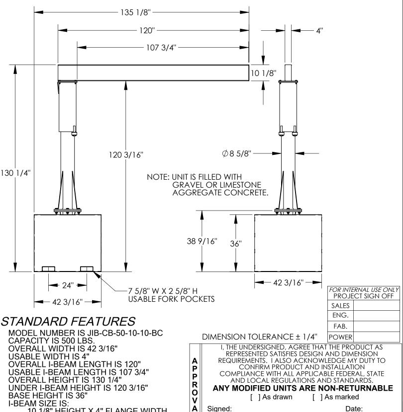
10 1/8" HEIGHT X 4" FLANGE WIDTH FORK CENTERS IS 24" **USABLE FORK POCKETS IS:** 7 5/8" W X 2 5/8" H UNIT WEIGHT IS 5,947 LBS. APPROX. DURABLE LIQUID PAINT BLUE FINISH
