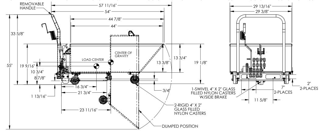
NEVER EXCEED LOAD CENTER RATING PER FORK TRUCK MANUFACTURER'S GUIDELINES. DO NOT USE THIS FORK TRUCK ATTACHMENT IF LOAD WILL EXCEED FORK TRUCK MANUFACTURER'S LOAD CENTER RATING. APPROX. WEIGHT/LOST LOAD=209.23 LBS.
