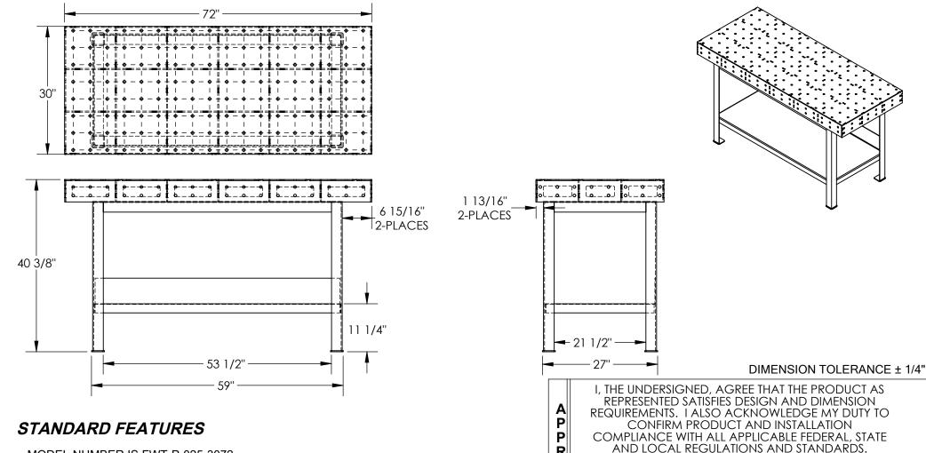
MODEL NUMBER IS FWT-P-025-3072 OVERALL WIDTH IS 72" USABLE WIDTH IS 72" **OVERALL LENGTH IS 30" USABLE LENGTH IS 30"** OVERALL HEIGHT IS 40 3/8" MAX CAPACITY IS 8,000 LBS HOLES FOR USE WITH Ø5/8" AND 16mm TOOLS DECK THICKNESS IS 1/4" TABLE TOP HOLE SPACING IS 4" X 4" TABLE SIDE HOLE SPACING IS 2" X 4" UNPAINTED STEEL CONSTRUCTION
