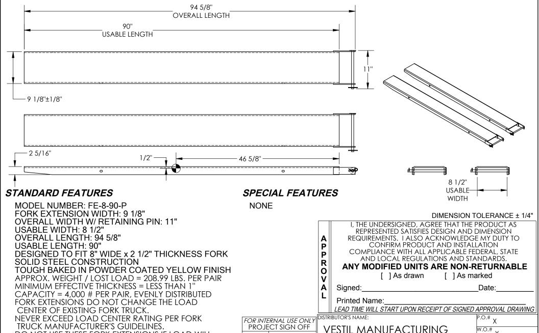
EXCEED FORK TRUCK MANUFACTURER'S LOAD CENTER RATING. FORK EXTENSIONS MUST NOT EXCEED 150% ORIGINAL FORK LENGTH
